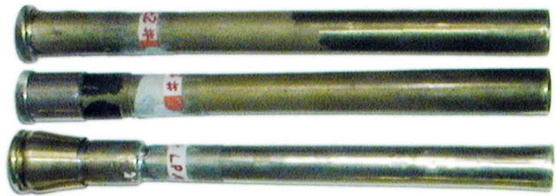
Figure 3: Three different leadpipes for a rotary trumpet.
